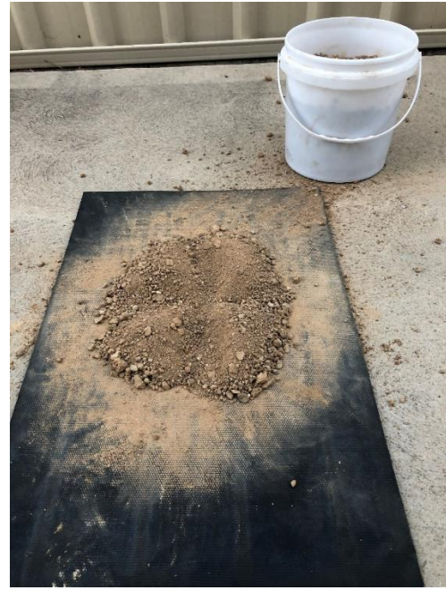
Figure 6.5: Cone and quartering.
