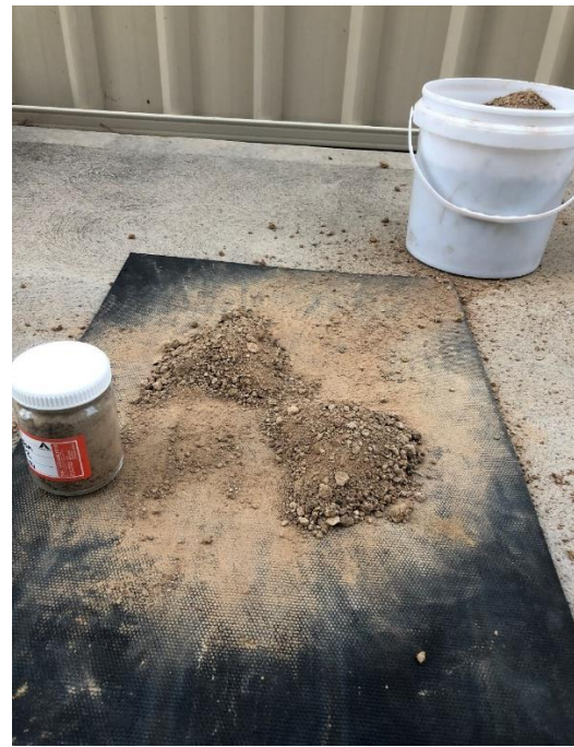
Figure 6.6: Sample volume reduction.
