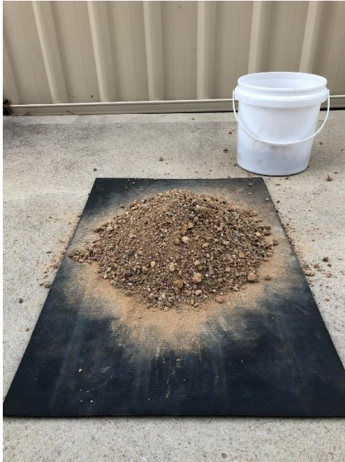
Figure 6.5: Cone and quartering.
