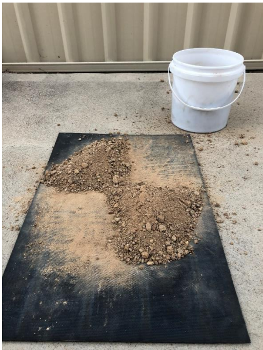
Figure 6.6: Sample volume reduction.
